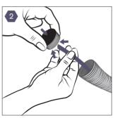
Push the cable lying in the pipe through the KABSEAL CAP membrane.
