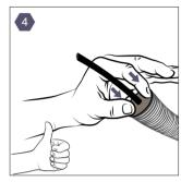
Push the KABSEAL CAP into the pipe.
