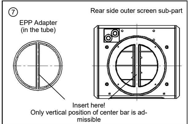
Fasten the outer screen sub-part using the screws enclosed! Place the cover on top!!
