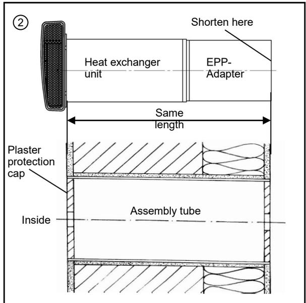
Insert the fan unit (inner housing sub-part, heat exchanger unit and EPP adapter) into the assembly tube!
