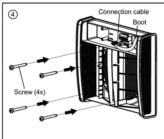
Insert the connection cable through one of the boots of the inner housing sub-part in the section of electrical connection! Fasten the inner housing sub-part to the wall using the screws enclosed!
