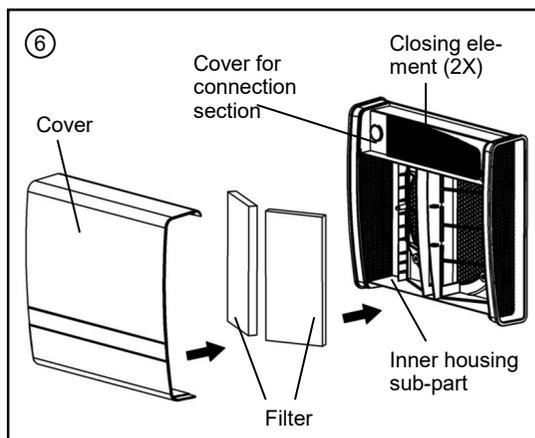
Mount the cover for the electrical connection section and insert the closing element on top!
