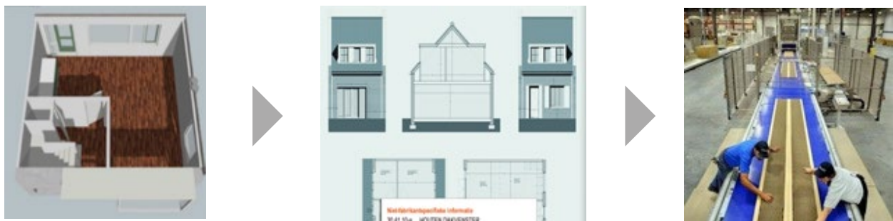
3D scanning, BIM generates technical drawings based on existing concepts, flexible factory makes prefab solutions
